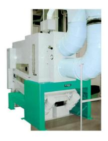
Thickness grading for a uniform parboiling result - No over-boiled or under boiled grains
